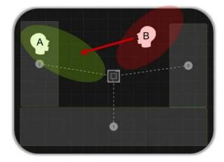
The Virtual Acoustic Boundary relies on DSP, which means it can behave differently under different conditions. It will deliver the most improvement in medium to large rooms where there is some space between pickup lobes and in rooms without many reflective surfaces like glass or concrete that can make it harder for the algorithm to localize sound sources. The feature is adjustable to suit different situations.
